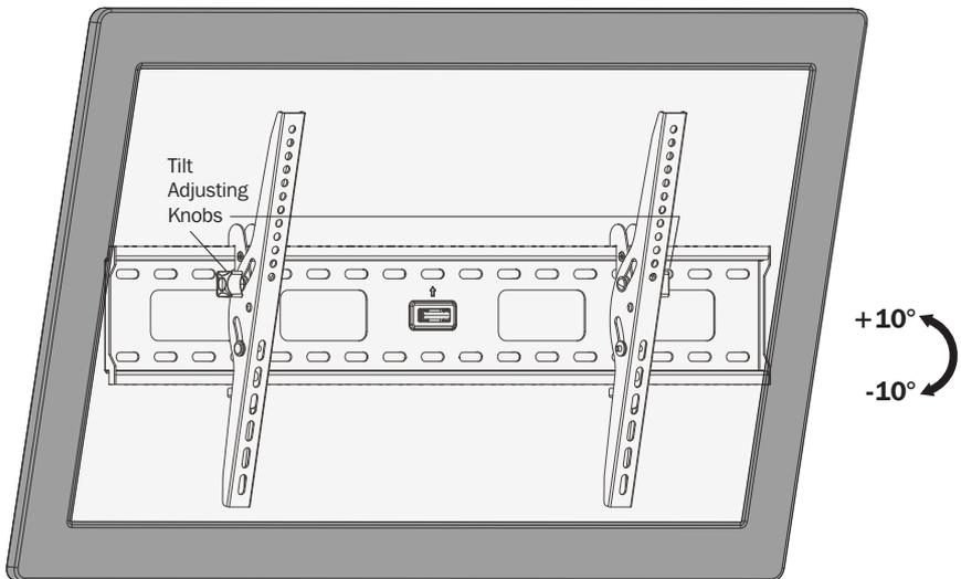
To adjust the tilt angle, loosen the Tilt Adjusting Knobs located on the sides of the adapter brackets. Once the display is at the desired angle, retighten the knobs to hold.
