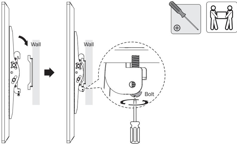
Using an assistant or mechanical lifting equipment, hook the display with attached adapter brackets over the top of the mounted wall-plate. Tighten the two bolts on the bottom of the adapter brackets to secure the unit.
