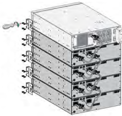
240V EBM connection to 8000VA and 11000VA UPS
