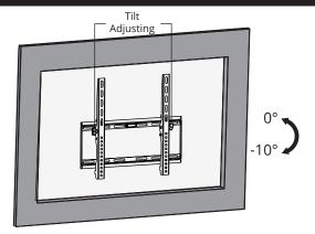
To adjust the tilt angle, loosen the Tilt Adjusting Knobs located on the sides of the adapter brackets. Once the display is at the desired angle, retighten the knobs to hold.
