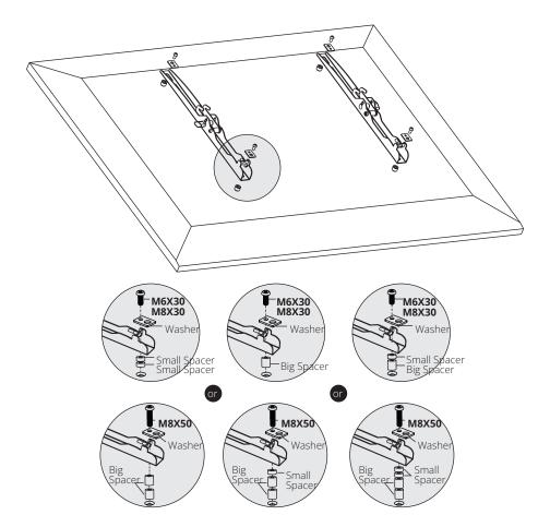
**Note:** Choose appropriate screws, washers and spacers (if necessary) according to the type of screen.
